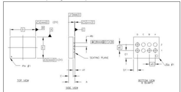
Note: Dimension b is measured at the maximum solder bump diameter, parallel to primary datum C.
