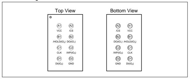
Figure 1d.Ball Assignments, 8-ball WLCSP (Package Code BY)
