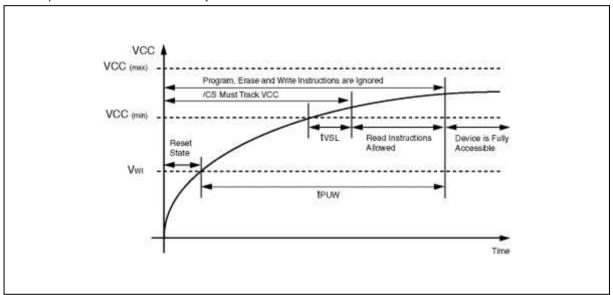
Figure 40a. Power-up Timing and Voltage Levels
