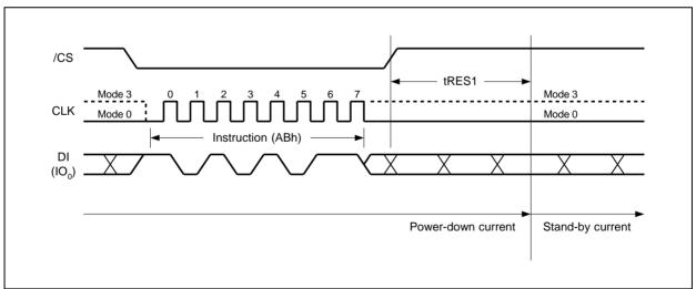
Figure 28a. Release Power-down Instruction Sequence
