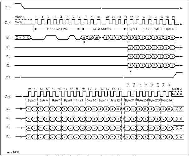
Figure 20. Quad Input Page Program Instruction Sequence Diagram
