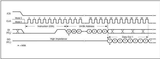
Figure 9. Read Data Instruction Sequence Diagram
