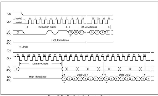
Figure 10. Fast Read Instruction Sequence Diagram
