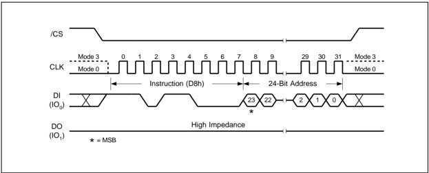
Figure 23. 64KB Block Erase Instruction Sequence Diagram
