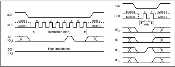
Figure 6. Write Disable Instruction Sequence Diagram
