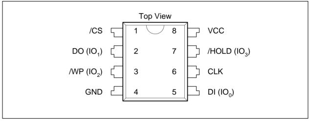
Figure 1c.Pin Assignments, 8-pin PDIP (Package Code DA)
