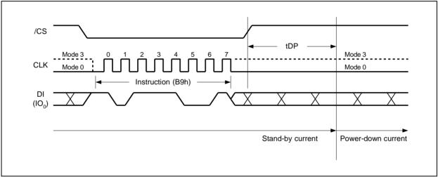
Figure 27. Deep Power-down Instruction Sequence Diagram
