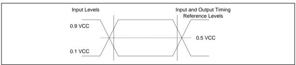
AC Measurement I/O Waveform
