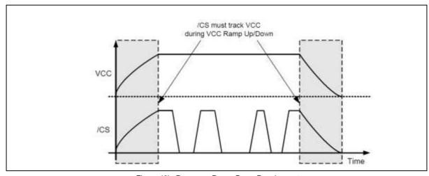
Figure 40b. Power-up, Power-Down Requirement
