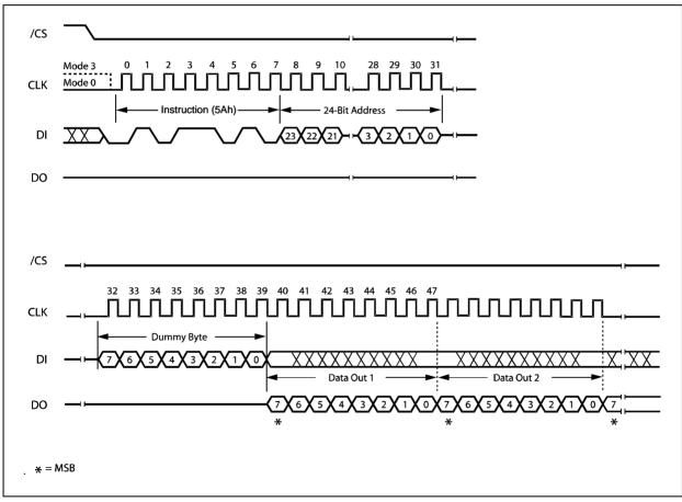
Figure 34b. Read SFDP Register Instruction Sequence Diagram
